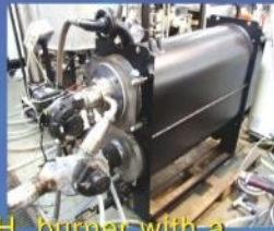
Prototype H 2 burner with a condensing boiler (60 kWth)
